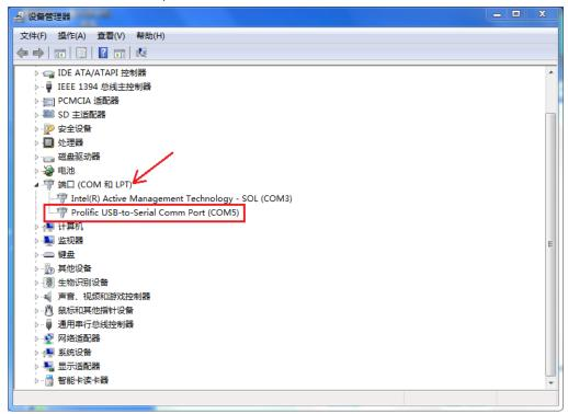
3. Run the FPE1.38 program. After selecting the serial number of USB-to-SerialPort at the "SET" icon, the state of the serial port is changed from red to green. At this time, the other end of the
